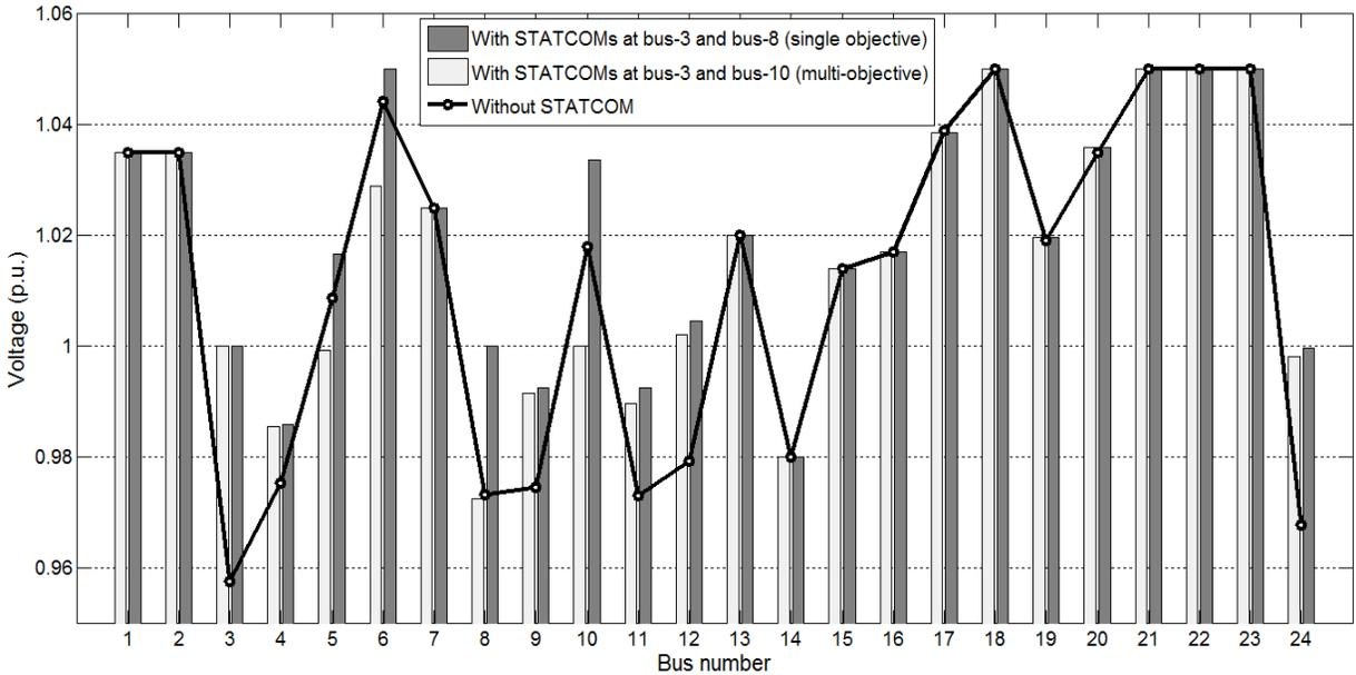
Fig. 5: Voltage profile of IEEE 24-bus system without STATCOM and with STATCOMs at bus-3, bus-10 (multi-objective) and STATCOMs at bus-3, bus-8 (single objective) at a loading factor of 0.3 p.u.
