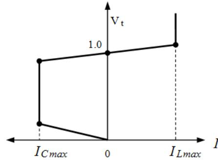
Fig. 2: V-I characteristic of STATCOM
