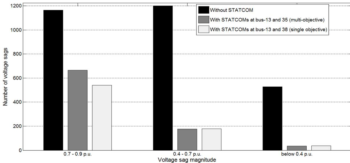
Fig. 7: Overall voltage sags in different voltage ranges without STATCOM and with STATCOMs at bus-13, bus-35 (multi-objective) and with STATCOMs at bus-13, bus-38 (single objective) in IEEE 57-bus system for symmetrical fault
