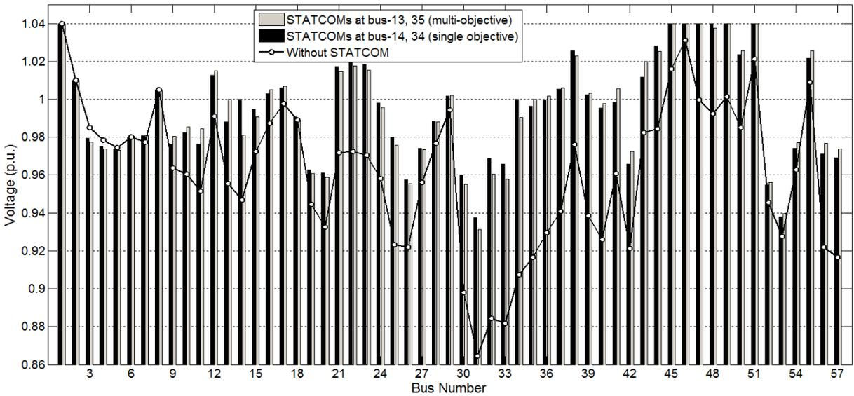
Fig. 8: Voltage profile of IEEE 57-bus system without STATCOM and with STATCOMs at bus-13, bus-35 (multi-objective) and with STATCOMs at bus-14, bus-34 (single objective) at a loading factor of 0.2 p.u.
