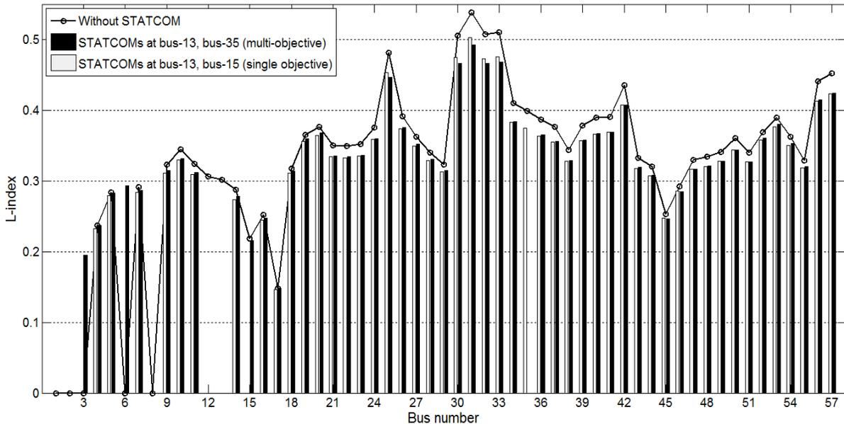
Fig. 9: L index at various buses in IEEE 57-bus system without STATCOM and with STATCOMs at bus-13, bus-35 (multi-objective) and with STATCOMs at bus-13, bus-15 (single objective) at a loading factor LF = 0.2 p.u.
