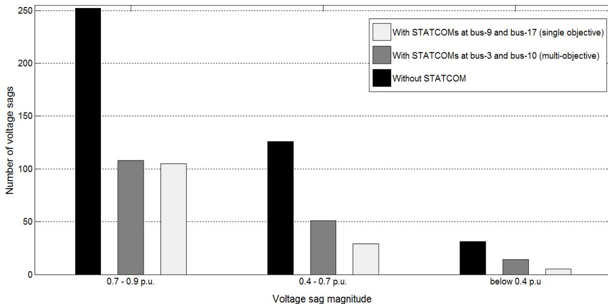
Fig. 4: Overall voltage sags in different voltage ranges without STATCOM and with STATCOMs at bus-3, bus-10 (multi-objective) and with STATCOMs at bus-9, bus-17 (single objective) in IEEE 24-bus system
