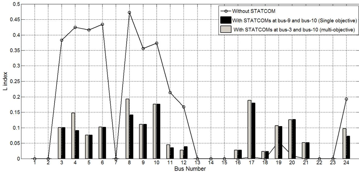
Fig. 6: L index at various buses in IEEE 24-bus system without STATCOM and with STATCOMs at bus-3, bus-10 (multi-objective) and with STATCOMs at bus-9, bus-10 (single objective) at a loading factor LF = 0.3
