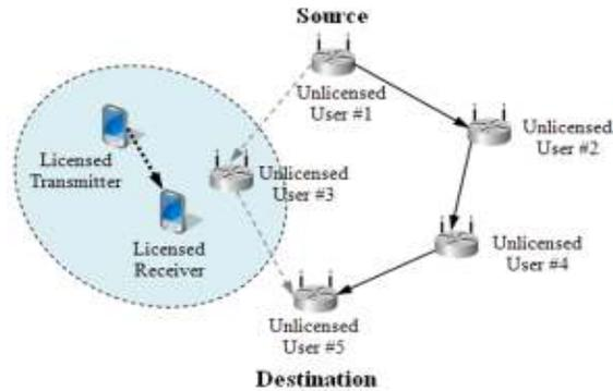
Fig. 2: Challenge on data routing in CRAHNs due to PU activity
