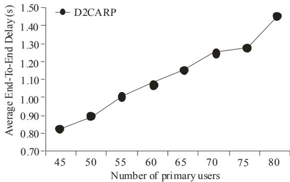
Fig. 10: Simulation results of average end-to-end delay against number of PUs
