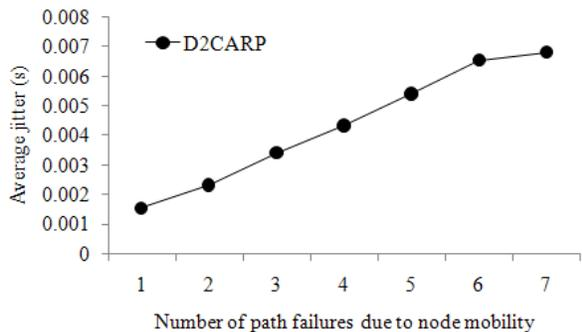
Fig. 11: Simulation results of average jitter against number of path failures due to node mobility
