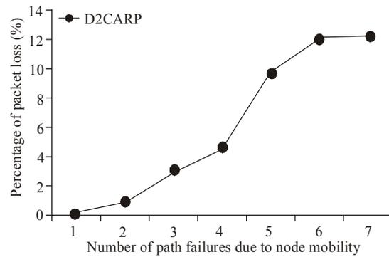
Fig. 7: Simulation results of percentage of packet loss against number of path failures due to node mobility
