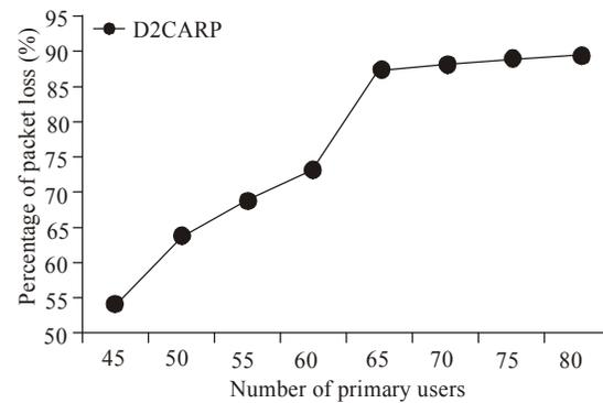
Fig. 8: Simulation results of percentage of packet loss against number of PUs
