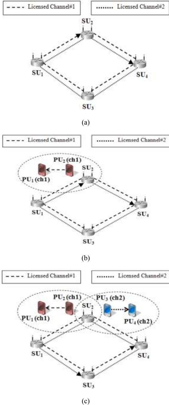
Fig. 4: Advantage of exploiting the joint path and spectrum diversity, (a) no PU activity is detected, (b) PU activity over channel 1 is detected, (c) PU activities over channel 1 and channel 2 are detected
