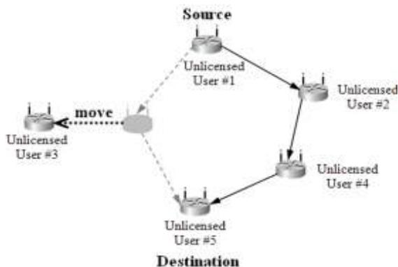
Fig. 3: Challenge on data routing in CRAHNs due to node mobility
