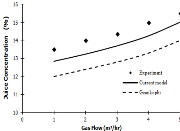
Fig. 9: Experiment and modeling data for falling film evaporation of sugarcane juice. The experiment was done at constant juice flow rate  $80 \text{ L/h}$  and initial concentration of 12%
