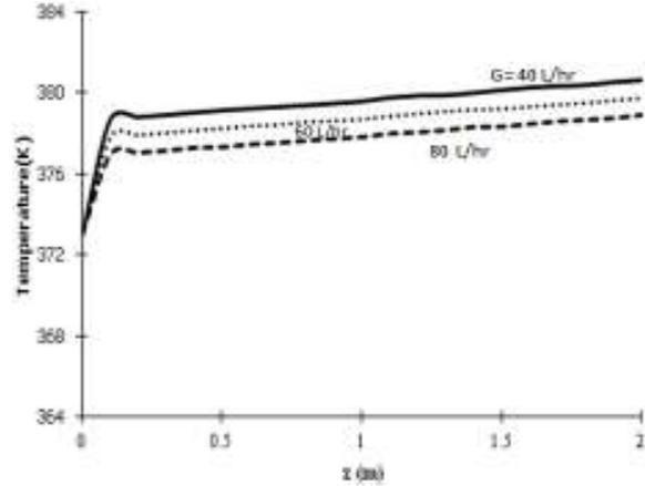
Fig. 4: Temperature profile of solution at the wall with gas flow rate of  $1 \text{ m}^3/\text{h}$  and initial concentration of 12%
