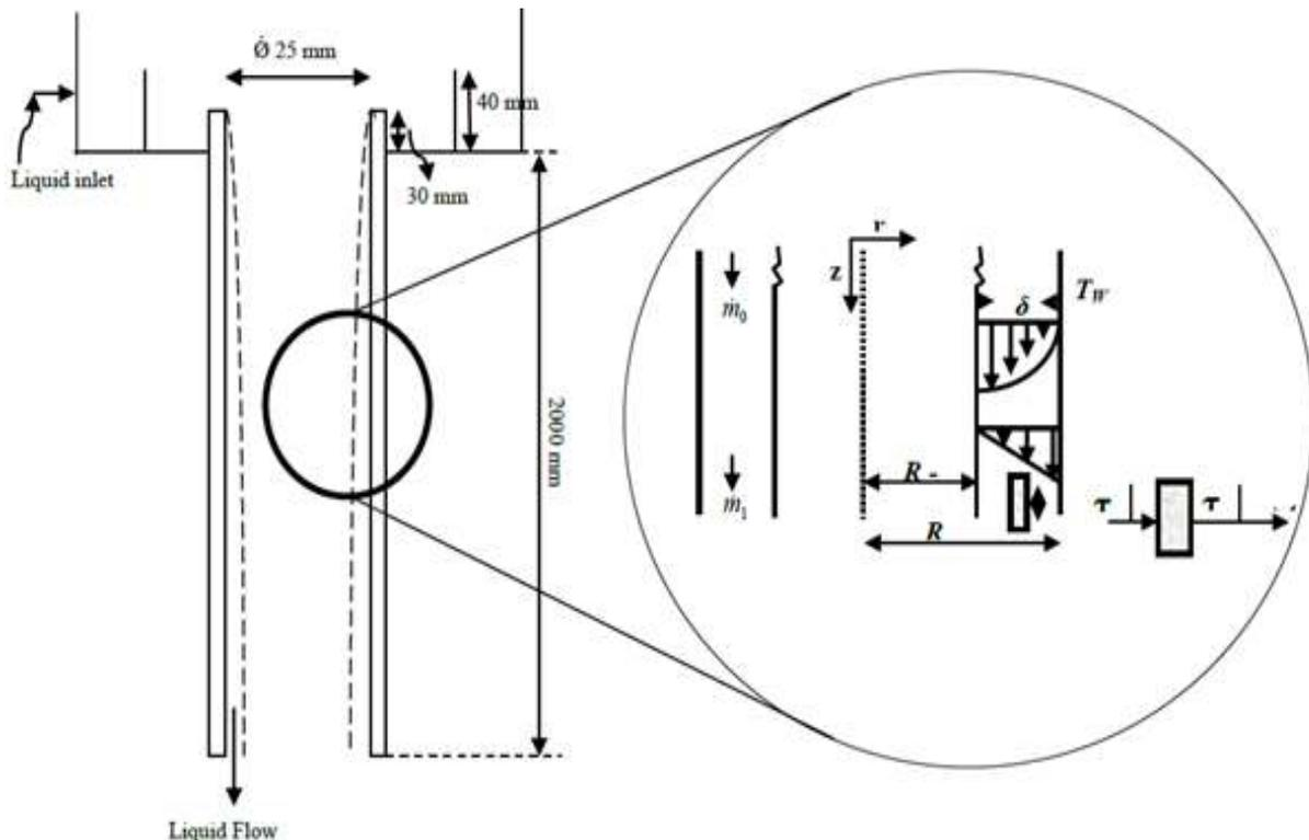
Fig. 1: Schematic diagram of vertical falling film evaporator
