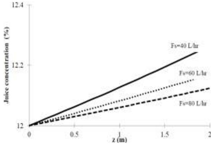
Fig. 7: Profile of juice concentration in tube at axial direction. The simulation was conducted at gas flow rate of  $1 \text{ m}^3/\text{h}$  and initial concentration of 12%
