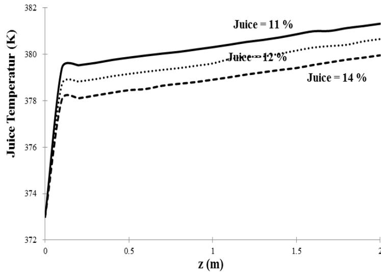
Fig. 5: Temperature profile of juice during evaporation at the axial direction as function of initial juice concentration. The simulation was conducted at juice solution of 40 L/h and gas flow rate of  $1 \text{ m}^3/\text{h}$
