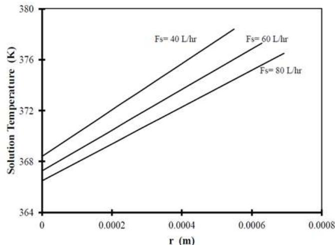
Fig. 2: Temperature distribution of solution with constant gas flow rate of 2 m<sup>3</sup>/h and initial concentration of 11%
