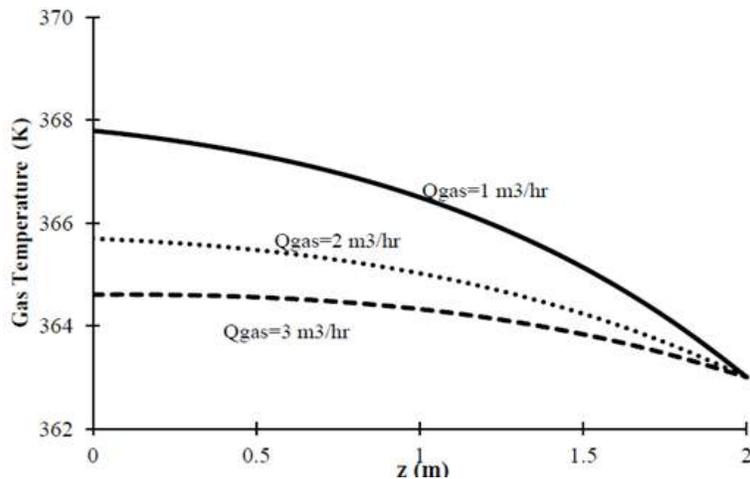
Fig. 6: The temperature profile of gas at the axial direction. The simulation was conducted at juice flow rate of 40 L/h and initial concentration of 12%
