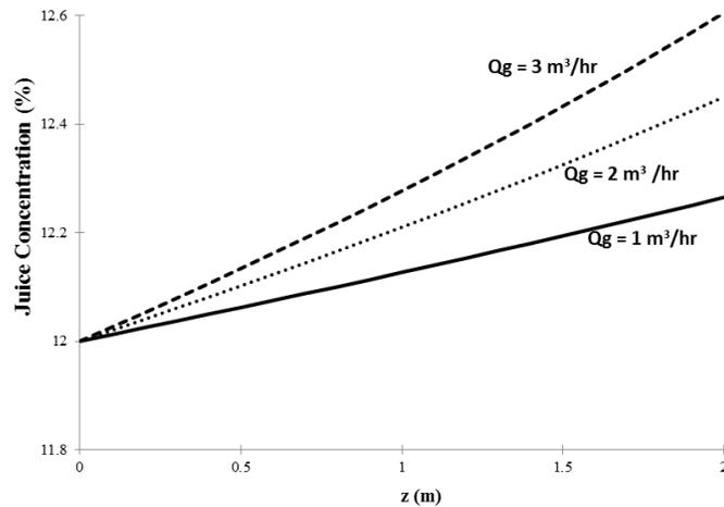
Fig. 8: Effect of gas flow rate to juice concentration. The simulation was done at constant solution flow rate  $40 \text{ L/jam}$  and initial concentration of 12%
