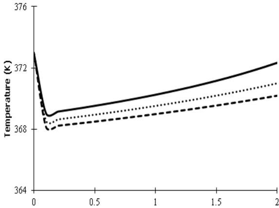
Fig. 3: Temperature profile at the interface for gas flow rate of  $1 \text{ m}^3/\text{h}$  and initial concentration of 12%
