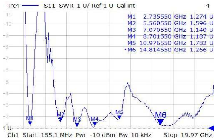
Fig. 11: VSWR vs. frequency of the proposed model
