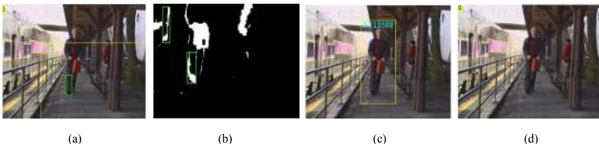
Fig. 4: Results of human and object detection in 10 th frame (Video); (a): Input frame; (b): Segmented output; (c): Detected human object with detection score; (d): Object detection
