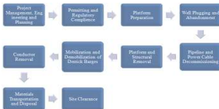
Fig. 3: Stages of offshore platform decommission (Proserv Offshore, 2010)
