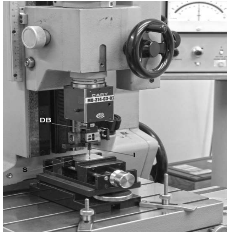
Fig. 2: Picture of indenter-specimen interaction; (DB): Device Body; (I): Indentator; (S): Specimen
