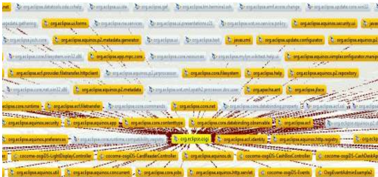
Fig. 2: Visual clutter caused by highly connected components
