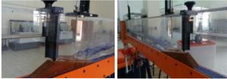
Fig. 2: Representation of the sill models and sluice gate
