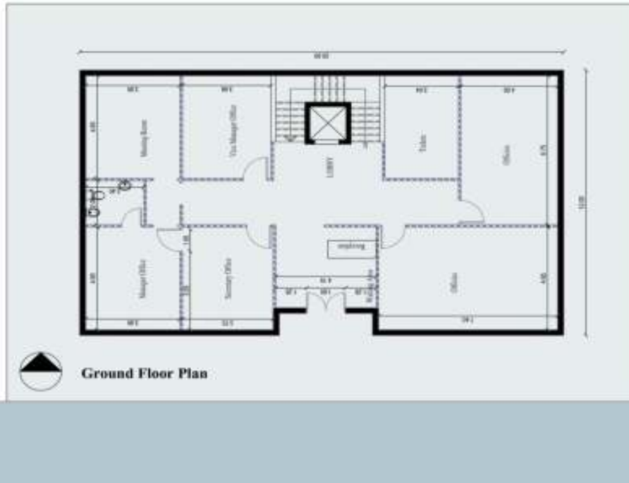
Fig. 4: Ground floor plan for the suggested of model, all the four floors are typical (Authors)
