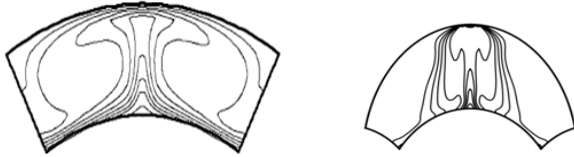
Fig. 3: Isotherms observed by Sarr (left) at Gr = 0.1 \cdot 10^7 and by us (right) at Ra = 10^7
