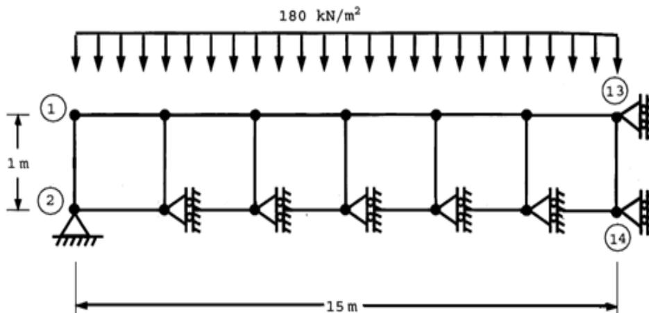
Fig. 5: Geometry and mesh of the elastoplastic cantilever beam
