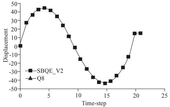
Fig. 4: Forced vibration of a rectangular solid 'displacements versus time-step'
