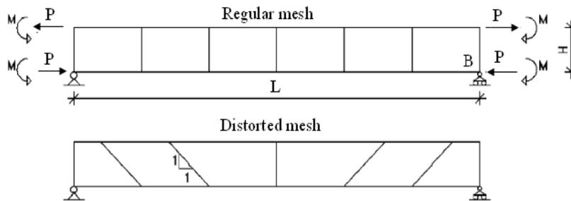
Fig. 7: Geometry and mesh of a simple beam
