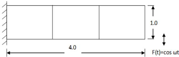
Fig. 3: Geometry and mesh of the cantilever beam subjected to forced vibration
