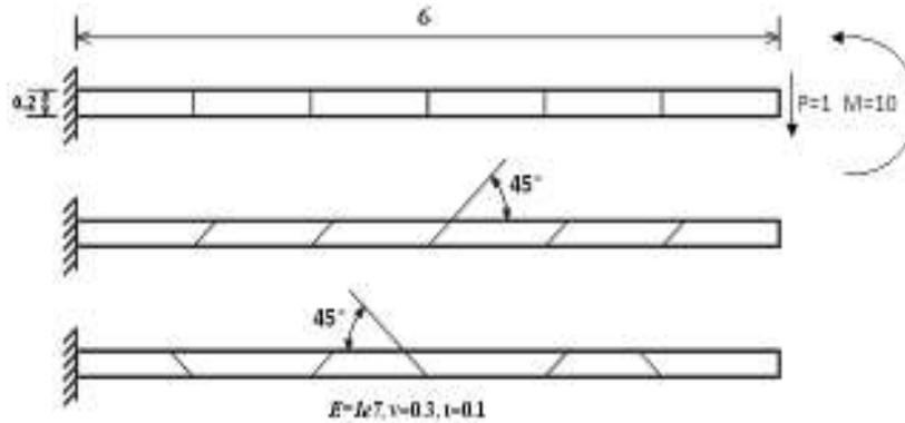
Fig. 6: MacNeal and harder patch tests: geometry, mesh and boundary conditions
