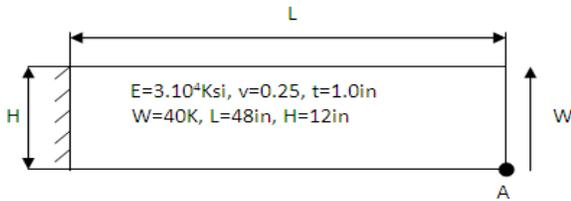
Fig. 8: Cantilever beam under a tip load
