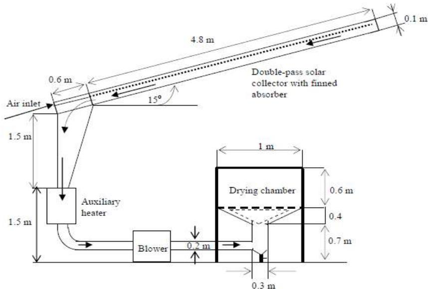
Fig. 9: Schematic diagram of solar assisted drying system
