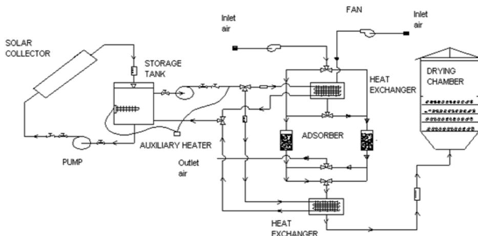
Fig. 24: Schematic diagram of solar assisted dehumidification system
