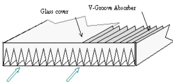
Fig. 15: Configuration of the V-groove absorber
