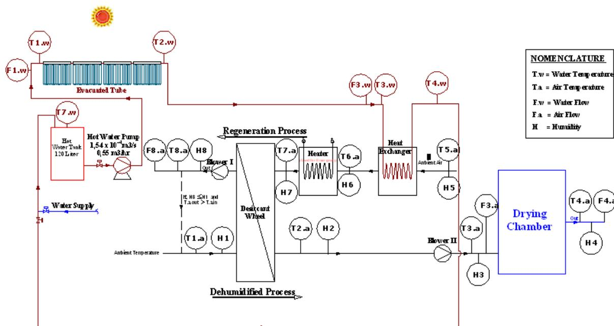
Fig. 26: Schematic diagram of solar desiccant dryer system
