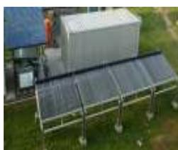
Fig. 27: Photograph of solar desiccant dryer system
