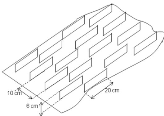
Fig. 12: Top view of the staggered fins absorber
