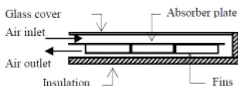
Fig. 11: The schematic double-pass solar collector with fins
