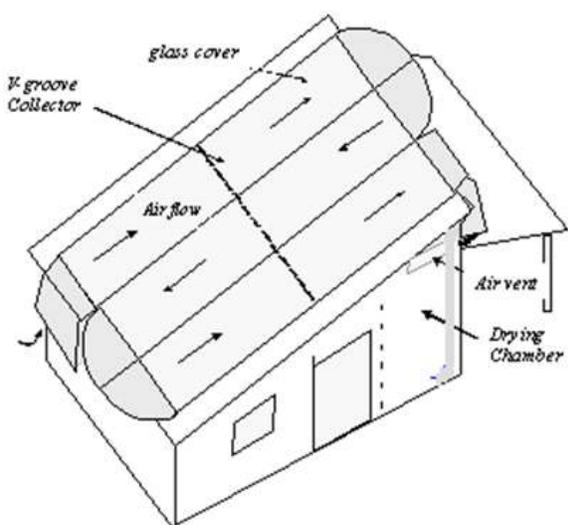
Fig. 14: Configuration of the solar dryer using V-groove absorber
