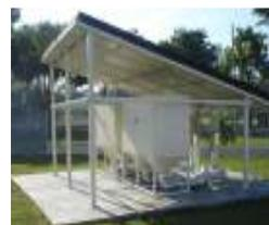
Fig. 13: Photograph of solar dryer using finned absorber
