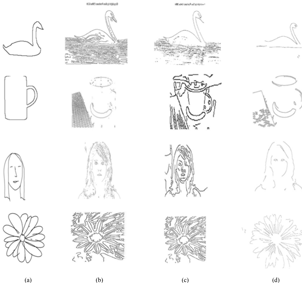
Fig. 4: (a) The sketch, (b) Sobel detector, (c) Canny with produce of multi scale, (d) Snake active boundary
