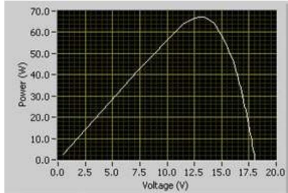
Fig. 7: Light current-voltage measurements from ~50 W<sub>p</sub> panel with two-mirror enhancement of peak power to ~70 W<sub>p</sub>
