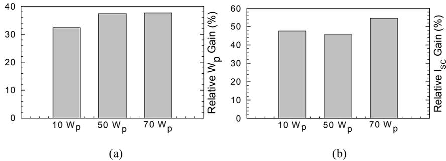
Fig. 8: Vertical bar-chart plot of percentage enhancement from three solar panels with output in 10-70 W<sub>p</sub> range; (a): Peak power; (b): Short-circuit current
