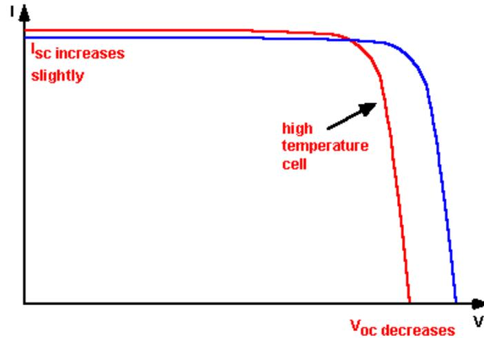
Fig. 5: Crystalline Si solar cell current-voltage response as a function of temperature
