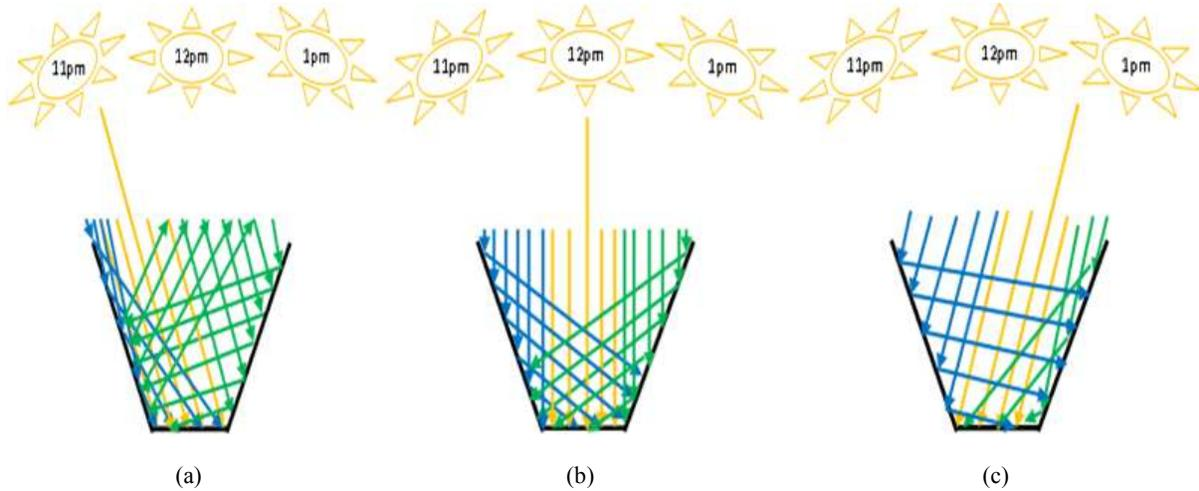
Fig. 1: Two-mirror Fresnel configuration for non-tracking system designed for operation during daylight hours from 11 AM to 1 PM (a-c)
