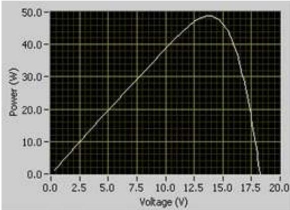
Fig. 6: Light current-voltage measurements from a 50 W<sub>p</sub> solar panel without mirror enhancement
