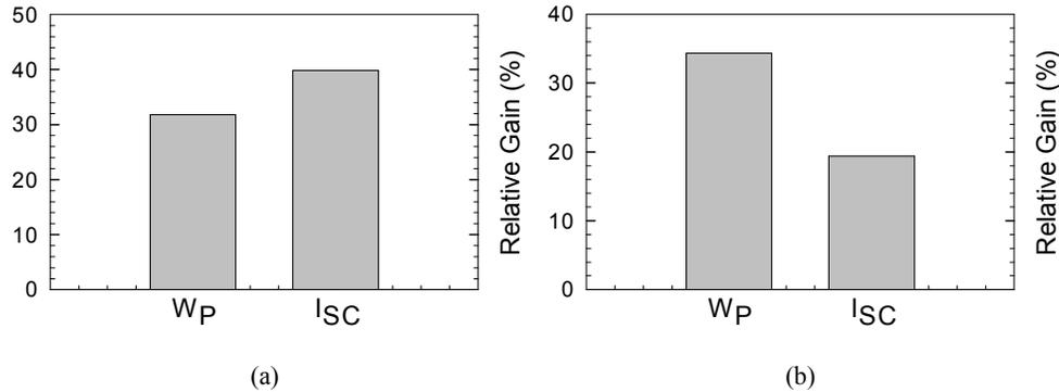
Fig. 10: Vertical bar plot for relative gains in; (a): 7  $W_p$ ; (b): 5  $W_p$  solar panels in tropical climate
