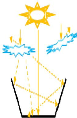
Fig. 4: Direct and diffused sunlight incident on a Fresnel mirror solar panel configuration
