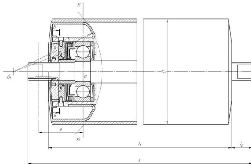
Fig. 2: Pipeline roller. 1 shell of a roller of the pipeline
