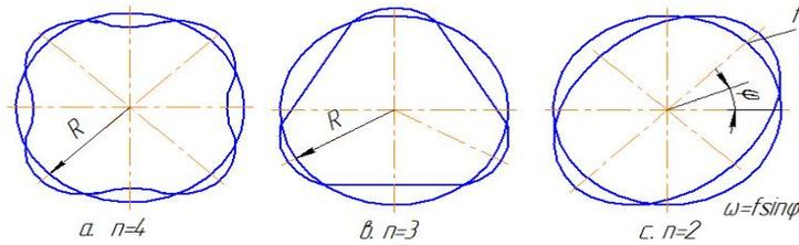
Fig. 3: Different kinds of distortions of the body from the roundness. A tetrahedron, in-cut, with oval
