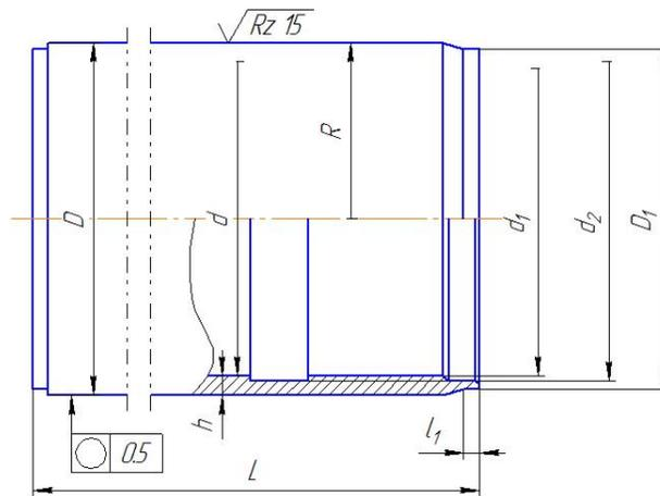
Fig. 1: Thin-walled casing of an underwater torpedo
