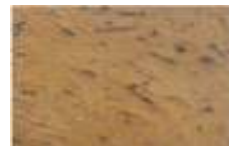
Fig. 4: Photography of a sample of mixture of clay of thiky, cow dung and copper
