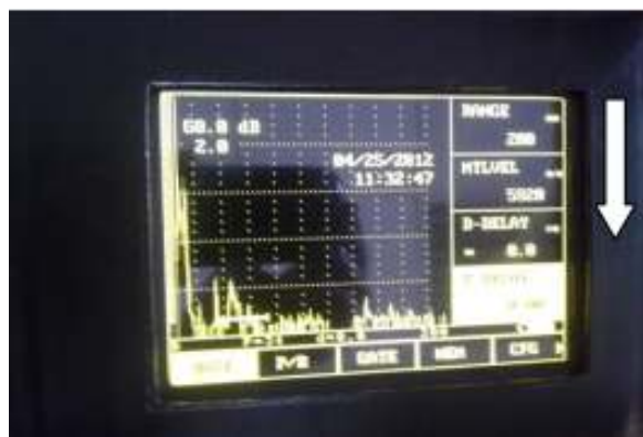
Fig. 15: An intermediate sign reflection shows on digital screen while inspecting 52.8% of wt. Ni-Ti sample made by powder-sand casting method
