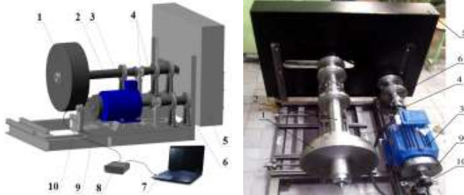
Fig. 5: The test bench for control of the mechanical efficiency of a chain transmission: 1: Loading rotary bodies; 2: Driven shaft; 3: Single-phase induction motor AIR 112MV6 (220/380 V), 1.1 kW, n = 940 rev/min; 4: Torque sensor M40-100; 5: Chain transmission casing; 6: Drive shaft; 7: PC with the installed software; 8: Registrating unit; 9: Reference body; 10: Encoder
