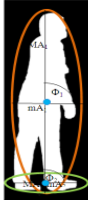
Fig. 2: Ellipse fitting model where MA 1 , MA 2 denotes major axes, mA 1 , mA 2 are minor axes and Φ 1 , Φ 2 are the orientation of horizontal and vertical ellipses
