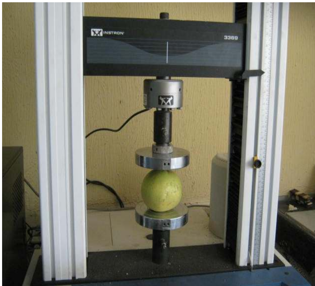
Plate 3: Grapefruit placed axially between parallel compression tools of the universal testing machine
