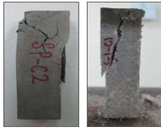
Fig. 2: Failure behaviours of compressive samples
