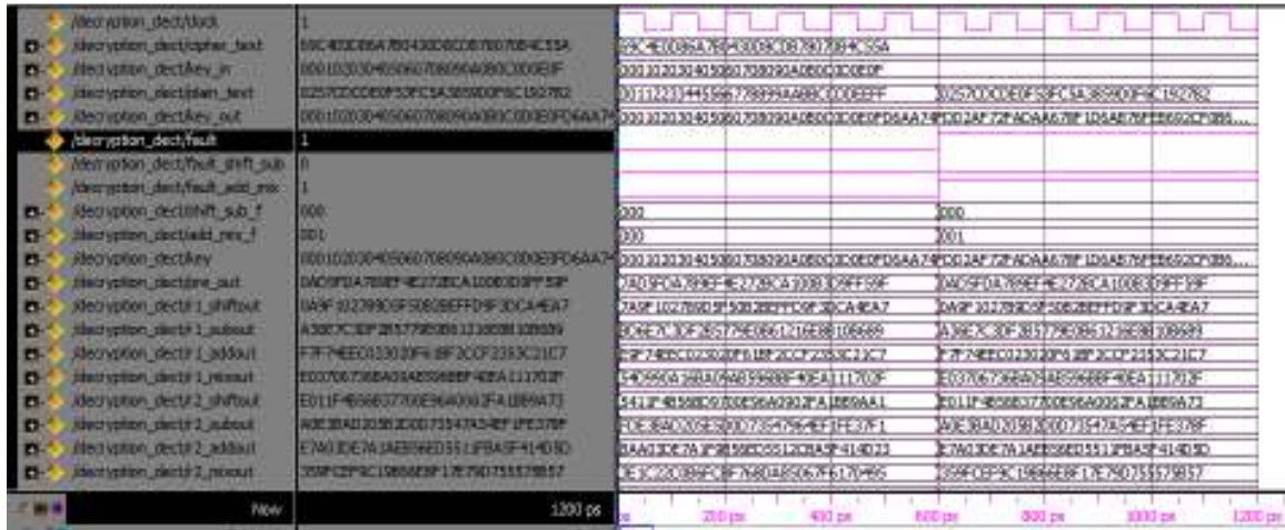
Fig. 6: Output of decryption for composite field s-box with error
