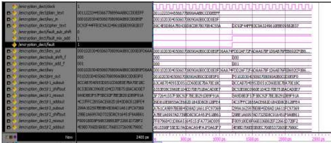
Fig. 3: Output of encryption for composite field s-box without error
