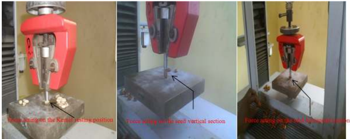
Fig. 3: Compressive tests for soursop seeds and kernels
