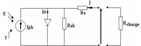
Fig. 2: Diagram of a real electric photovoltaic cell
