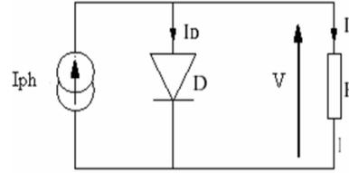
Fig. 1: Circuit diagram of an ideal solar cell
