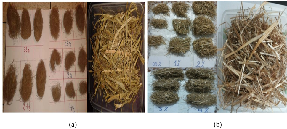
Fig. 2: (a): Pictures and the different masses of alfa used; (b): Pictures and the different masses of straw used
