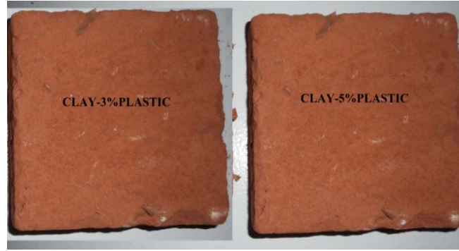
Fig. 3: View of the composite clay-plastic on different percentage of plastic
