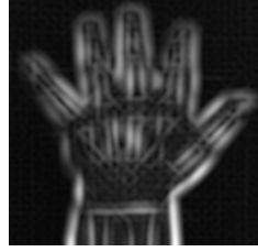
Fig. 8: Gabor wavelet transform feature extraction results for pre-processed images
