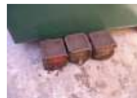
(c) Complete the compaction of cubes for compressive strength test
