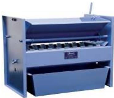
(a) Splitter for hematite ore sample preparation for sieve analysis
