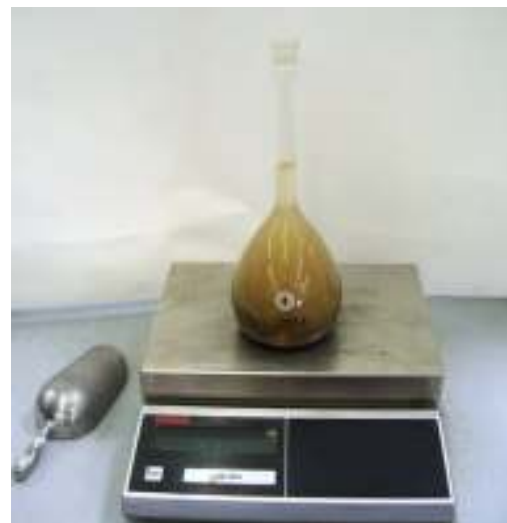
Fig. 7: Specific gravity testing
