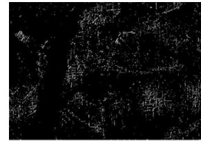
Fig. 2: After the crack detection using top-hat morphological transform
