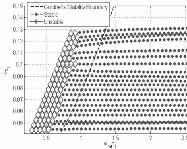
Fig. 6: The stability simulation results when  $v_{ctrl} > V_{DD}/2$  with symmetrical current  $I_p = i_p^{dn}$
