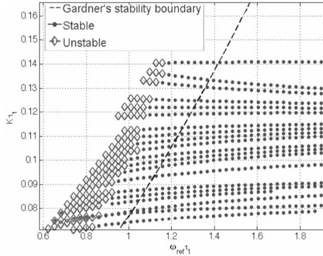
Fig. 5: The stability simulation results when  $v_{ctrl} = V_{DD}/2$  with symmetrical current  $i_p^{up} = i_p^{dn}$
