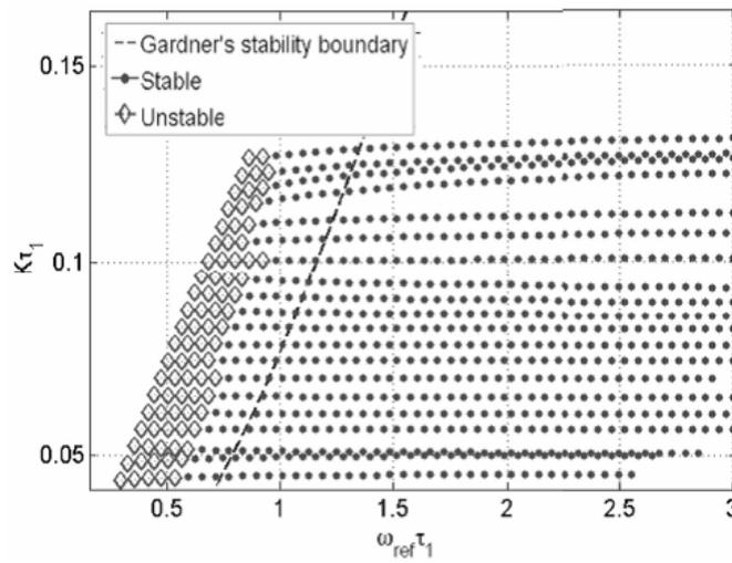
Fig. 8: The stability simulation results when  $v_{crr} < V_{DD}/2$  with symmetrical current  $I_p = i_p^{up}$
