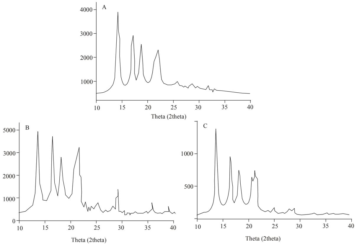
Fig. 4: XRD for; (A): neat PP; (B): 5%CaCO<sub>3</sub>; (C): 10%CaCO<sub>3</sub> nanocomposite at 25 rpm
