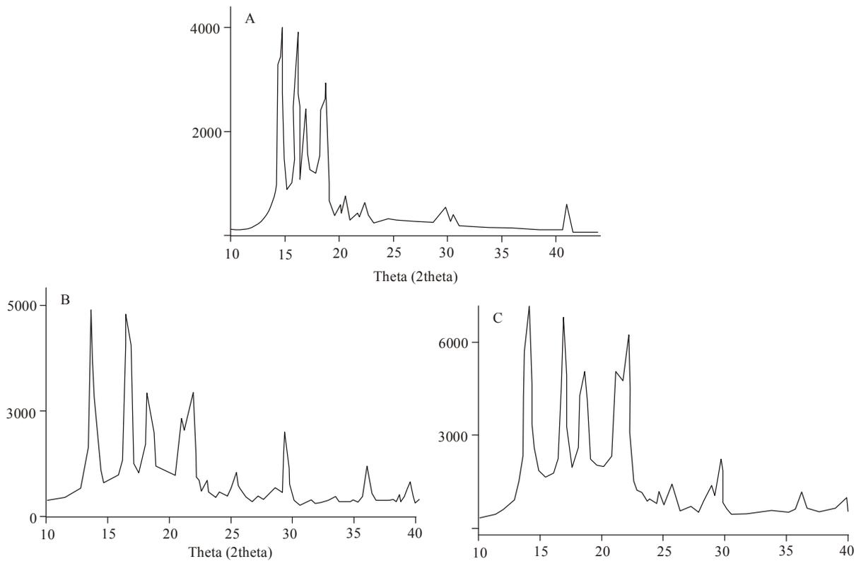
Fig. 5: XRD (A) waste PP, (B) 5%CaCO<sub>3</sub>, (C) 10%CaCO<sub>3</sub> nanocomposite at 25 rpm
