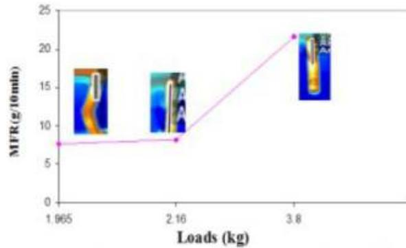
Fig. 9: The relation between melt flow rate and thermal images at different three loads
