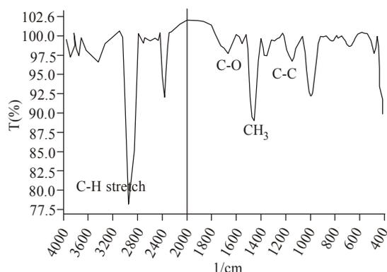
Fig. 3: FTIR for polypropylene
