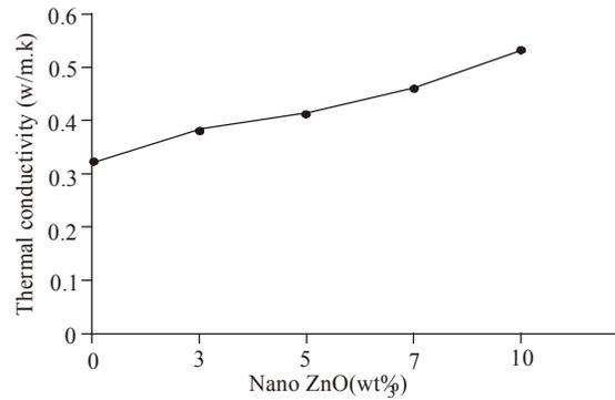
Fig. 8: Thermal conductivity behavior for waste PP with different ZnO nanoparticles concentration at 100°C
