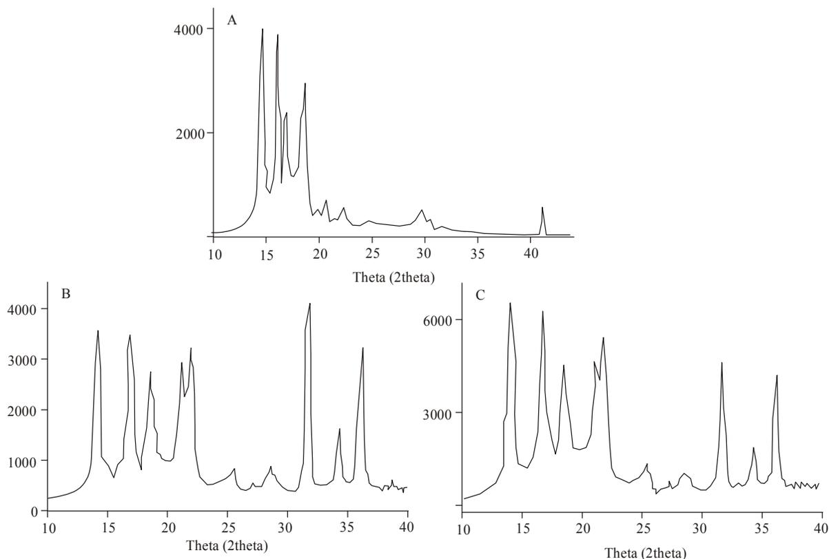
Fig. 6: The crystallinity level of nanocomposite; (A): neat waste PP; (B): 5% ZnO; (C): 10%ZnO nanoparticles
