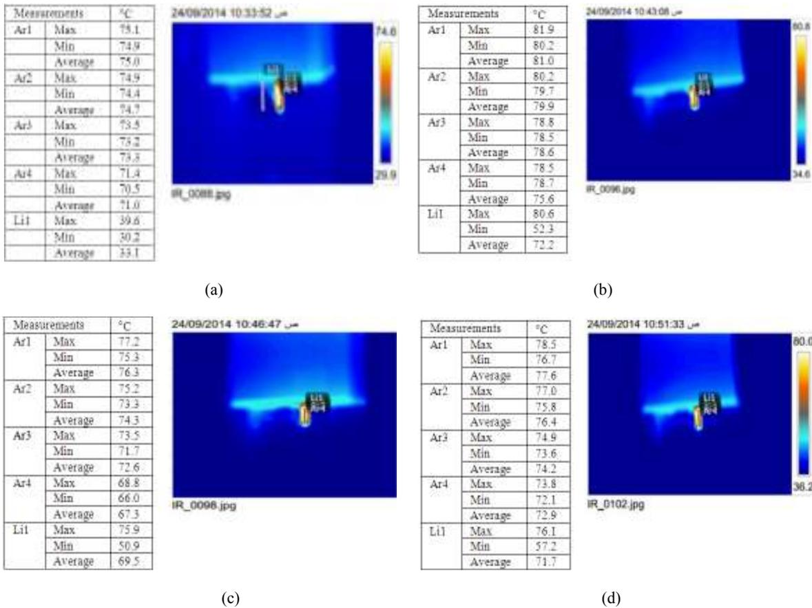
Fig. 11: Thermal image of virgin PP nanocomposite: - (A): 3%; (B): 5%; (C): 7% and; (D): 10wt% of CaCO<sub>3</sub> nanoparticles
