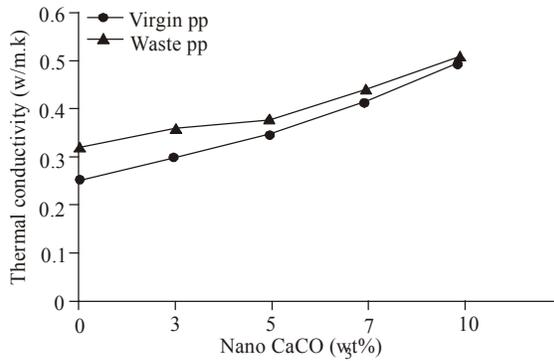
Fig. 7: Thermal conductivity behavior for virgin and waste PP with different CaCO<sub>3</sub> nanoparticles concentration at 100°C
