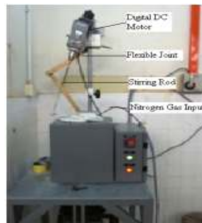
Fig. 2: Fabrication of metal matrix composite using the stir casting technique
