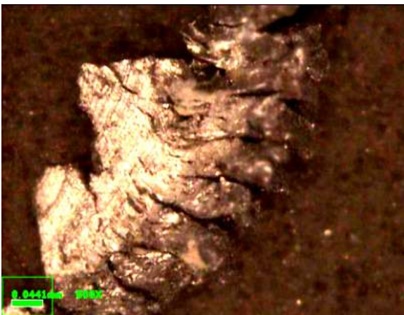
Fig. 7: Image for chip formation at cutting conditions V = 230 m/min; F = 0.8 mm/tooth; D.O.C 0.5 mm
