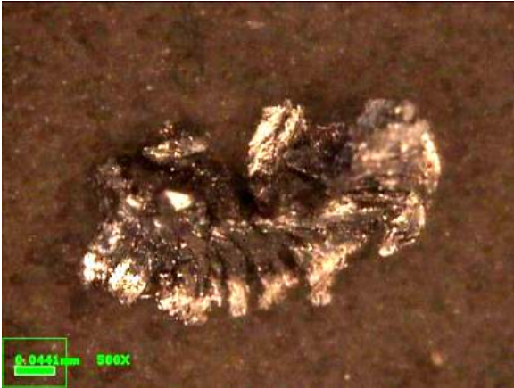
Fig. 5: Elemental chips on cutting conditions V = 230 m/min, F = 0.4 mm/tooth, D.O.C 0.4 mm
