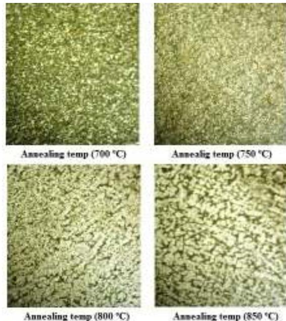
Fig. 5: The effect of annealing temperature on the homogeneity of AISI 3115 alloy steel structures, X200
