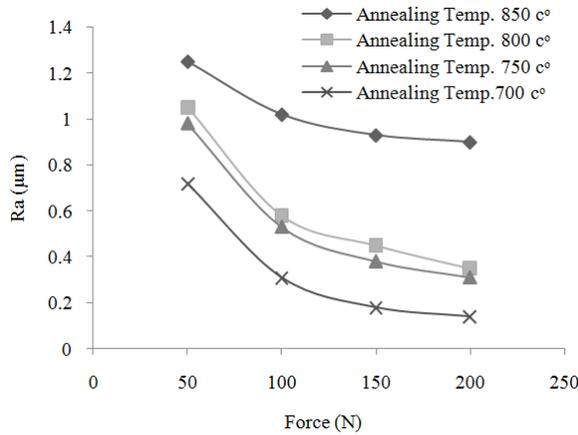
Fig. 9: The effect of the roller burnishing force on the average surface roughness of annealed AISI 3115 alloy steel (where the feed = 0.04 mm/rev and Spindle speed = 260 rev/min)
