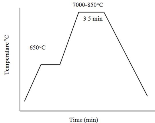
Fig. 1: Annealing regimes of AISI 3115 alloy steel
