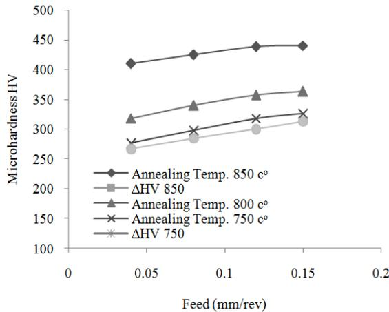
Fig. 7: The effect of the roller burnishing feed on the microhardness of annealed AISI 3115 alloy steel (where is the Force = 200 N and Spindle speed = 260 rev/min)
