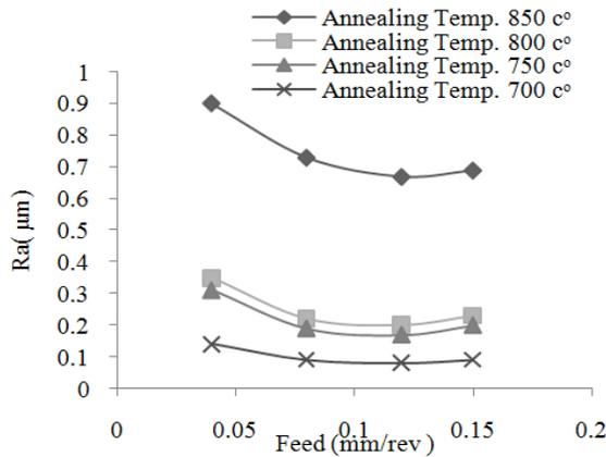
Fig. 10: The effect of the roller burnishing feed on the average surface roughness of annealed AISI 3115 alloy steel (where is the Force = 200 N and Spindle speed = 260 rev/min)
