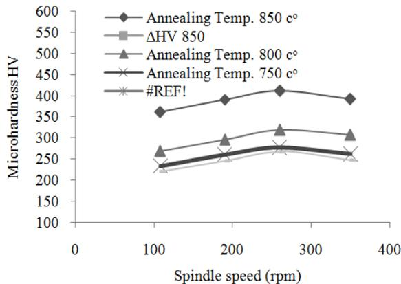
Fig. 8: The effect of the roller burnishing spindle speed on the microhardness of annealed AISI 3115 alloy steel where is the Force = 200 N and (feed = 0.04 mm/rev)
