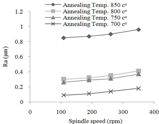
Fig. 11: The effect of the roller burnishing spindle speed on the average surface roughness of annealed AISI 3115 alloy steel (where is the Force = 200 N and feed = 0.04 mm/rev)
