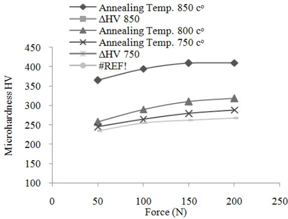
Fig. 6: The effect of the roller burnishing force on the microhardness of annealed AISI 3115 alloy steel (where is the feed = 0.04 mm/rev and Spindle speed = 260 rev/min)
