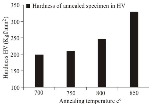
Fig. 4: The effect of annealing temperatures on hardness of AISI 3115 alloy steel
