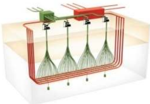
Fig. 10: American shale oil CCR process (United States Department of Energy & Office of Naval Petroleum and Oil Shale Reserves, 2014)
