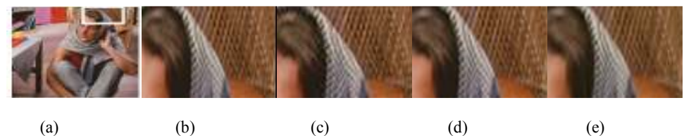
Fig. 11: Part of the reconstructed color Barbara image sample, the compression parameters are taken and highlighted in Table 8; (a): Original color Barbara image; (b): Original; (c): JPEG; (d): JPEG2000; (e): Proposed system
