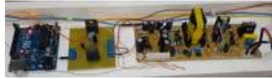
Fig. 7: Close view for the motor drive circuit and controller
