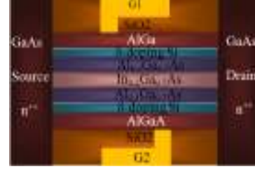
Fig. 1: Structure of double gate field plate \text{In}_{0.2}\text{Ga}_{0.8}\text{As}/\text{Al}_{0.3}\text{Ga}_{0.7}\text{As} HEMT including double hetero-structure
