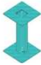
Fig. 5a: Mesh of columns SC & SW
