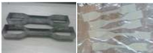
Fig. 1: Tension test specimen of biopolymers films of cassava starch
