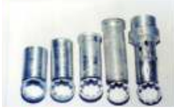
Fig. 5: SAMPLES of internally- spline sleeves and cross section of it's at various cross in-feed
