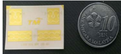
Fig. 14: Photograph of the fabricated planar SIW BPF and compact SIW BPF at 38GHz
