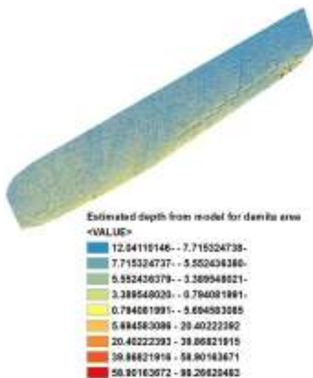
Fig. 7: Predicted bathymetry map for Damietta coastal area
