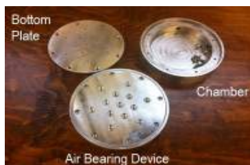
Fig.4: Air-bearing device components
