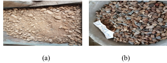
Fig. 1: Photos of the alluvial gravel 0/31.5 (a) before and (b) after washing
