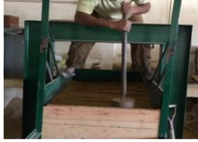
Fig. 9: Preparation of comacted sand / (sand +5% silica fume) backfill layers
