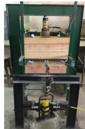
Fig. 2: Overview of the pull-out testing model
