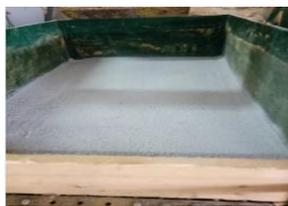
Fig. 7: Prepared graded sand with 5% silica fume
