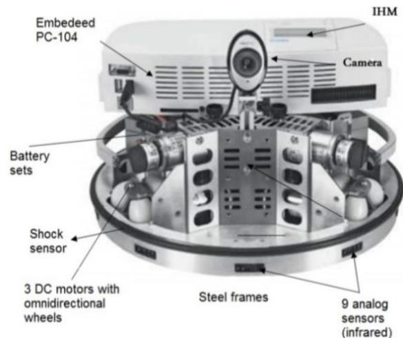
Fig. 1: Robotino<sup>MD</sup> an omnidirectional mobile robot (Weber and Bellenberg, 2010)
