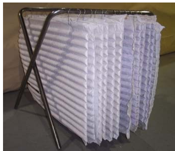
Fig. 4: Absorption curtain used for carbon dioxide
