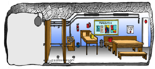
Fig. 1: Arrangement of permanent refuge chamber
