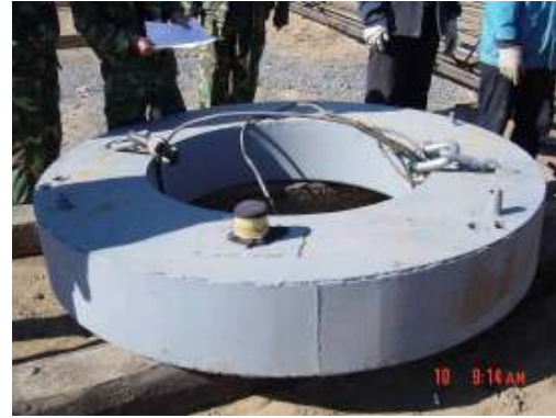
Fig. 2: Load cell of Longhua Bridge
