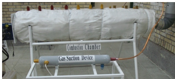
Fig. 1: Laboratory combustion chamber
